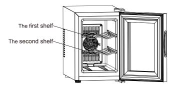
6. When the surrounding temperature is 25°C and the pantry has no load, it will take around 3.5 hours to decrease the pantry 's temperature from 25°C to 17°C.
